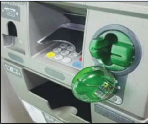
Criminals capture debit card data by affixing fake skimmers like this one over the top of ATM slots.
