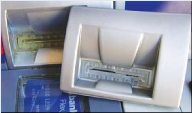
Criminals capture debit card data by affixing fake skimmers like this one over the top of ATM slots.
