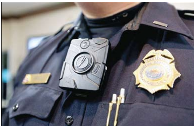
The cameras CPD uses are Axon Body 2 devices made by a division of the company that makes TASER weapons. They can record high-definition video for at least 12 hours and up to 70 hours at lower resolutions. The video can be uploaded to the cloud and viewed on a mobile phone. Audio can be muted. Courtesy Loop North News
