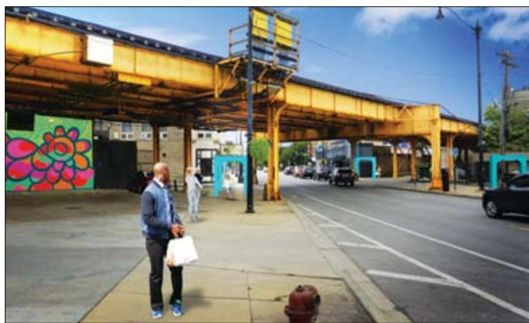
The Arches are coming to Lincoln Ave. just south of Wrightwood, and will include four illuminated archways featuring integrated LED sensors that activate a dynamic light display when people and CTA trains pass by.
