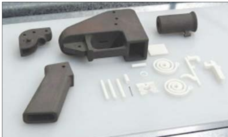
The Liberator, a plastic 3-D printed gun, disassembled.
