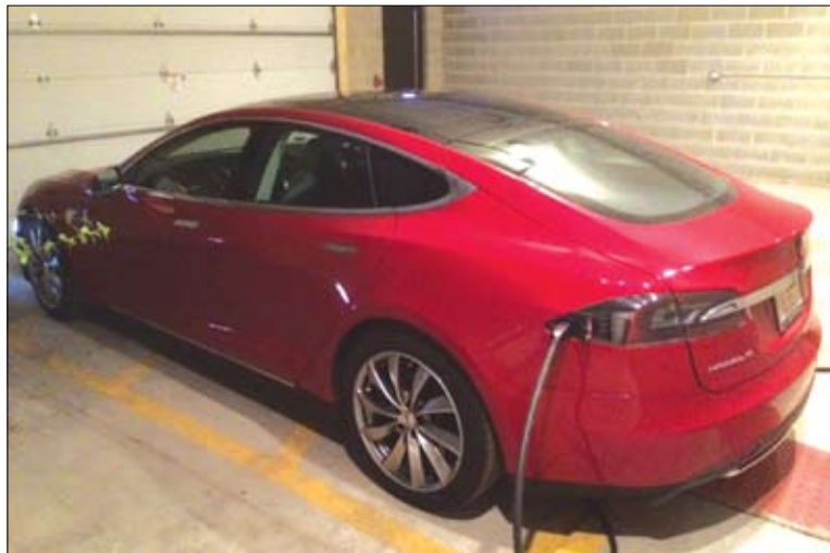
The Tesla High Power Connector adds 58 miles per hour.
