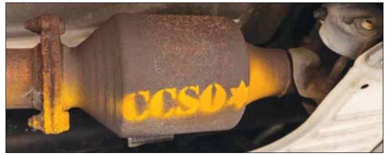
An etched VIN number will allow law enforcement to trace a recovered stolen catalytic converter back to the owner, potentially increasing the chance for criminal charges.
