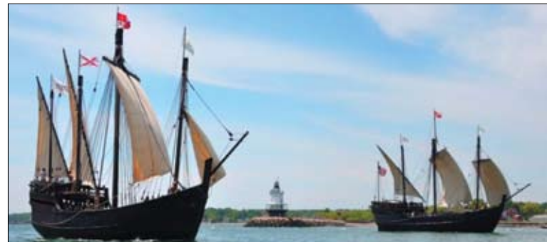
The Nina (left) had a deck length of 65 feet and a sail area of 1919 sq. ft. The Pinta had a deck length of 85 feet and a sail area of 3800 sq. ft.
